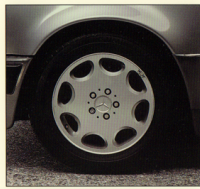
The 500E rides on new eight-hole 16-inch light-alloy wheels.
